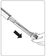
**D6** The shock absorber kit is now free. Remove the kit and the whole suspension line.
