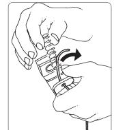
R6 Wrap the suspension line around the support arm (see section D1) to relieve the tension. Tie a new knot on the mark and attach the plastic cover to hide the knot.
