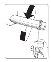
**D2** Extend the suspension line and hold it there by winding it around the support arm.
