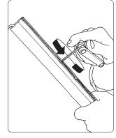
**D5** Remove the two screws which hold the shock absorber kit.
