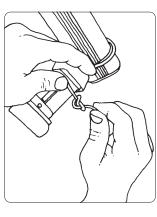
**D3** Detach the snap lock by untying the knot and let the line go in.
