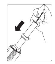
R3 Continue to feed the coil spring tool into the support arm from below over the line wheel.
