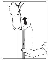
R1 Unpack your shock absorber kit. Attach the suspension line to the coil spring tool. Feed the coil spring tool into the back support bar from below. Pull the new shock absorber kit in place.
