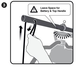
Adjust the ropes. You want to be able to tilt the gimbal without the top handle, monitor or batteries touching the EasyTilt.
