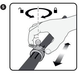
To adjust the ring side-to-side, you can release the ring by turning the lever counter clockwise. To get it centered on the EasyTilt fasten it between the two tracks.
