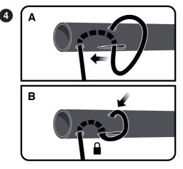
**A.** Fasten the ropes by pressing them into the declining track of the EasyTilt.
