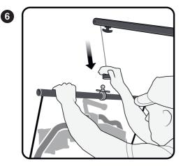
Fasten your Easyrig onto the EasyTilt by using the ball stud with our Quick Release or simply slide the ring to the side and use our standard camera hook. You are now ready to shoot!
