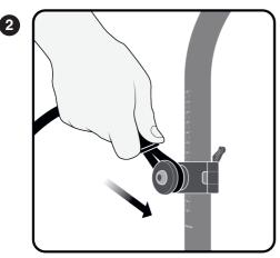
Align the loop over the dedicated track on the spindle and fasten it by pressing the sealing ring forward. Balance the gimbal by turning the spindle forward or backwards
