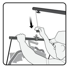
Fasten your Easyrig onto the EasyTilt by using the ball stud with our Quick Release or simply slide the ring to the side and use our standard camera hook. You are now ready to shoot!
