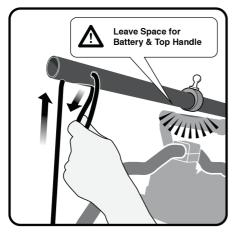
Adjust the ropes. You want to be able to tilt the gimbal without the battery or top handle touching the EasyTilt.
