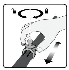
To adjust the ring side-to-side, you can release the ring by turning the lever counter clockwise. To get it centered on the EasyTilt fasten it between the two tracks.
