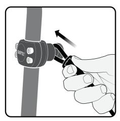
Align the loop over the dedicated track of the spindle link and fasten it by pressing the sealing ring forward.
