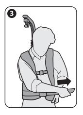
**Fig. 3**Put on your Easyrig 3 CINEMA. Adjust the hip belt until you find the rig comfortable. Pull the belt tightly.
