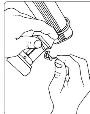
**D3** Detach the snap lock by untying the knot and let the line go in.
