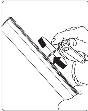
**R2** Fasten the new shock absorber kit with the two screws.
