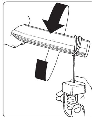
**D2** Extend the suspension line and hold it there by winding it around the support arm.
