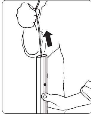
**R1** Unpack your shock absorber kit. Attach the suspension line to the coil spring tool. Feed the coil spring tool into the back support bar from below. Pull the new shock absorber kit in place.
