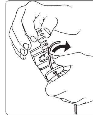
**R6** Wrap the suspension line around the support arm (see section D1) to relieve the tension. Tie a new knot on the mark and attach the plastic cover to hide the knot.
