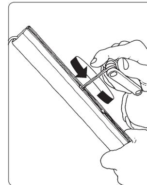
**D5** Remove the two screws which hold the shock absorber kit.
