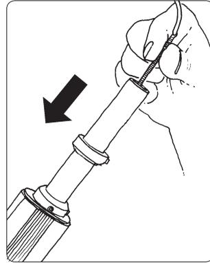
**R3** Continue to feed the coil spring tool into the support arm from below over the line wheel.
